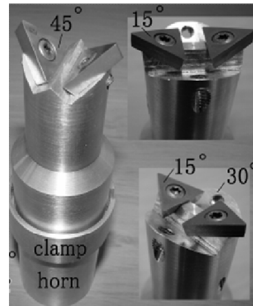
Fig. 5. Tooling system (horns and inserts) providing obliquity in vibrational oblique turning.
