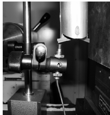
Fig. 6. Eddy current setup (measuring the vibrations amplitude of cutting tool tip).
